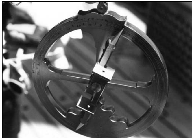
The projection of the sunbeam on the second pinule, after crossing the first one.
