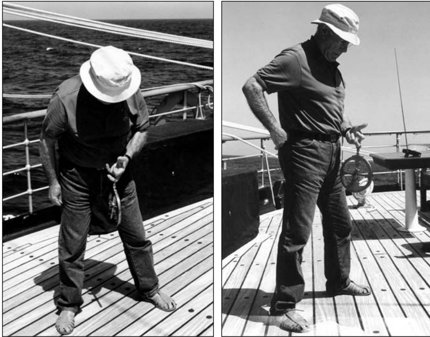
The plane of the instrument should be in the vertical plane of the sun. Note in the first photograph that the shade of the instrument in the deck indicates that it is in the same vertical plane of the sun.
